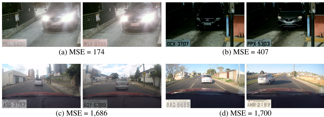
Figure 9.4: Two pairs of the most similar images (in terms of MSE) from distinct subsets from each of the RodoSol-ALPR (a, b) and UFPR-ALPR (c, d) datasets. In each pair, the left image belongs to the training set, while the right one belongs to the test set. Observe that LPs from different images captured by static cameras may be quite resembling. We show a zoomed-in version of the LP in the lower left region of each image for better viewing.
