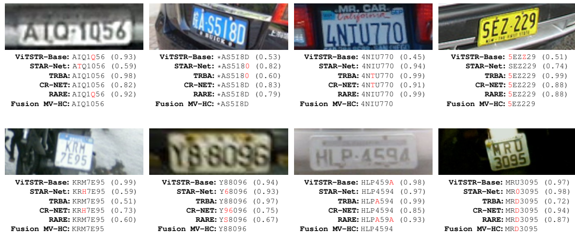
Figure 6.3: Predictions obtained in eight LP images by multiple models individually and through the best fusion approach. Although we only show the predictions from the top 5 models for better viewing, it is noteworthy that in these particular cases, fusing the top 8 models (the optimal configuration) yielded identical predictions. The confidence for each prediction is indicated in parentheses, and any errors are highlighted in red.
