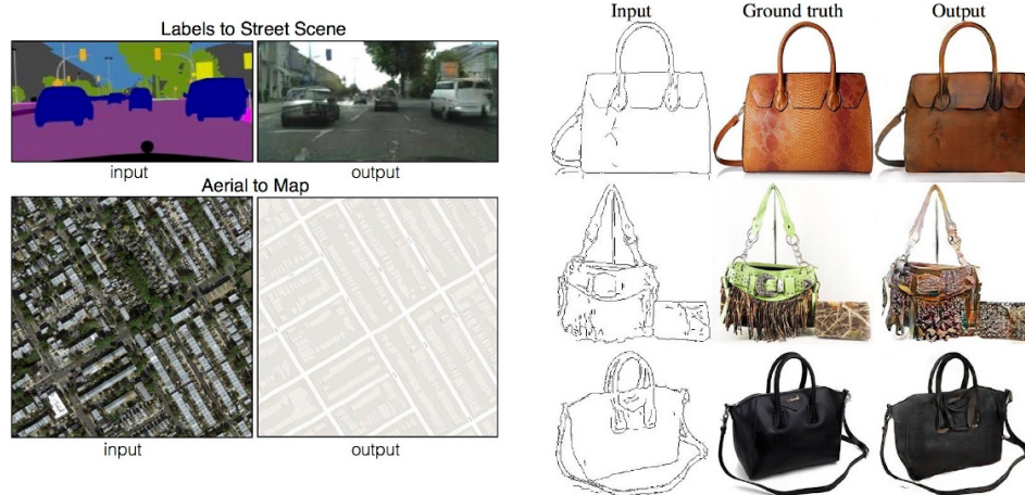
Figure 2.18: Image-to-image translation is a concept introduced by Isola et al. (2017) that encompasses many kinds of transformations of an image: converting segmentation masks into images, converting aerial photos into maps, converting sketches into photorealistic images, among others. Image adapted from (Isola et al., 2017).
