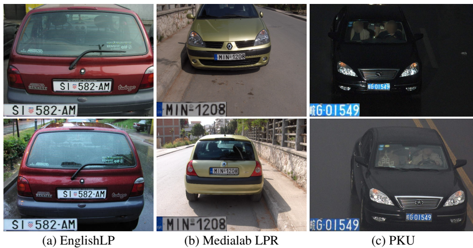
Figure 8.5: ALPR datasets that do not have a well-defined evaluation protocol are customarily divided into training and test sets randomly without the authors noticing that the same vehicle/LP may appear in multiple images. Above, we show a pair of near-duplicates from each of the EnglishLP, Medialab LPR, and PKU datasets. Observe that it is common for an LP to look very similar in different images even without rectification. We show a zoomed-in version of the rectified LP in the lower left region of each image for better viewing.
