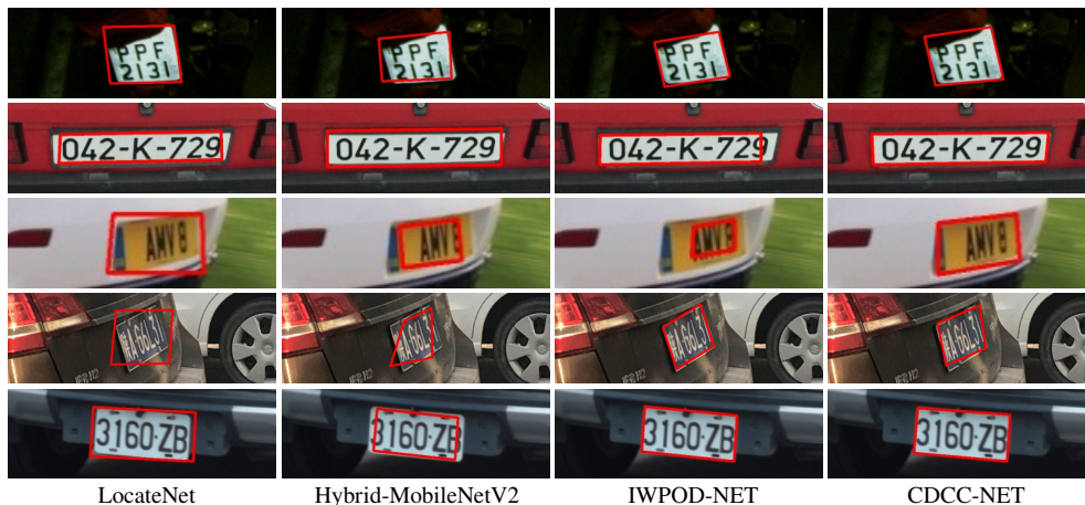
Figure 7.6: Qualitative results achieved by four different models in corner detection. For better viewing, we draw a polygon from the predicted corner positions.
