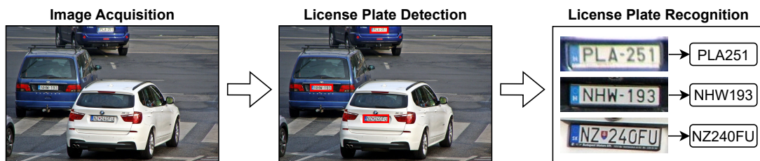
Figure 1.1: A typical ALPR system. It is divided into two stages: LPD and LPR. The former stage refers to locating the LPs within the input image, while the latter refers to identifying the characters on those LPs.
