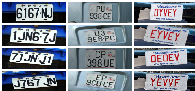
Figure 5.2: Illustration of the character permutation-based synthetic data generation method (Gonçalves et al., 2018) we adopted to reduce overfitting. The images in rows 2 to 4 were created based on the images shown in the top row.
