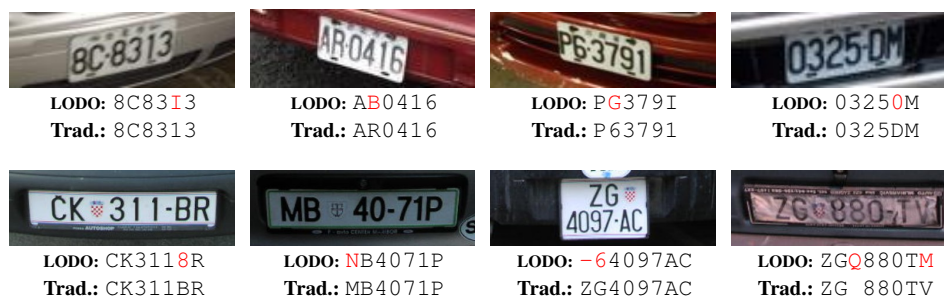
Figure 5.5: Comparison of the predictions yielded for the same LPs under the leave-one-dataset-out (LODO) and traditional-split (Trad.) protocols. The top row shows the predictions returned by ViTSTR-Base for four LPs from the AOLP dataset, while the bottom row shows the predictions made by STAR-Net for four LPs from EnglishLP. In general, the errors under the LODO protocol (outlined in red) were not observed in challenging cases (e.g., blurry or extremely tilted images). This suggests that these errors likely stemmed from differences between the training and testing data distributions.
