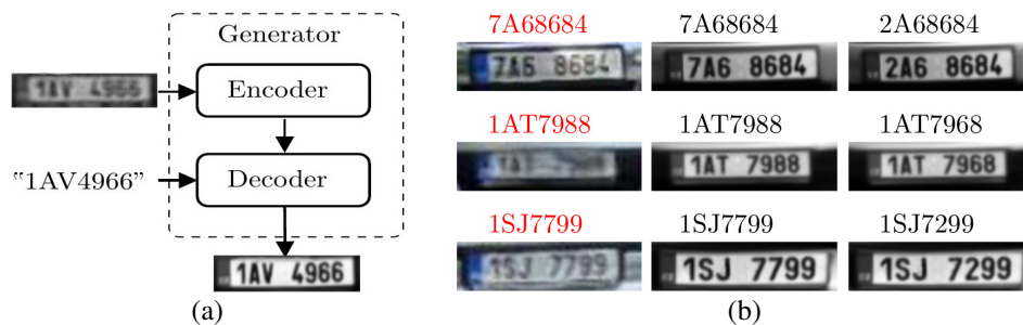
Figure 3.25: Vašek et al. (2018) proposed a super-resolution CNN-based generator that converts input low-resolution images into their high-resolution counterparts closely matching the structure of the input LP. (a) shows a simplified view of the super-resolution generator; it takes as input the low-resolution LP image and the string to be depicted. (b) shows impressive examples of high-resolution LP images created by their generator. The first column shows low-resolution images (the red strings denote the ground truth), while the second and third columns show images produced by the generator. Image adapted from (Vašek et al., 2018).
