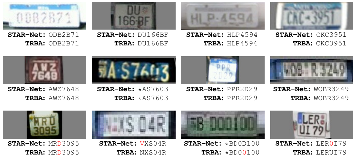
Figure 7.7: Predictions made for 12 LP images by STAR-Net and TRBA, the two models that exhibited the highest average performance in the intra-dataset experiments. Errors, if any, are highlighted in red. All LPs are well aligned because they were rectified before recognition, as detailed in Section 7.3.3.
