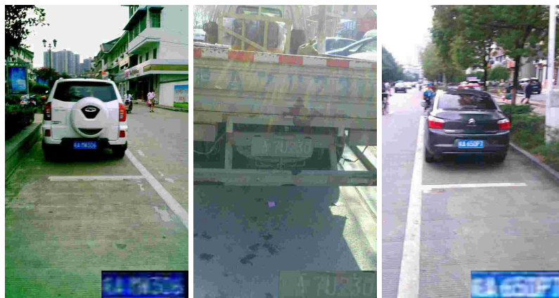
Figure 3.31: Three images that illustrate the high compression ratios in the CCPD dataset. As noted by Qiao et al. (2021); Silva and Jung (2022), it is clear that the high compression ratios impair the legibility of the LPs in some cases. We show a zoomed-in version of the vehicle’s LP in the bottom-right region of each image for better viewing.
