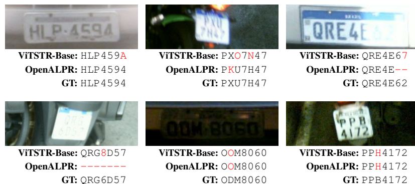
Figure 5.6: Some LP images from the RodoSol-ALPR dataset along with the predictions returned by ViTSTR-Base and OpenALPR. Observe that one character may become very similar to another due to factors such as blur, dirt, exposure levels (either too low or too high), rotations and occlusions. For correctness, we checked if the Ground Truth (GT) matched the vehicle make and model on the National Traffic Department of Brazil (DENATRAN) database.
