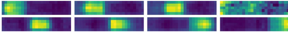
Figure 3.12: The attention of Holistic-CNN’s fully connected layers for different characters on a Czech LP. From left to right, top to bottom: 1st to 8th character. In most cases (i.e., on Czech LPs with less than eight characters), the 4th position does not contain any character (it is blank). Image reproduced from (Špaňhel et al., 2017).
