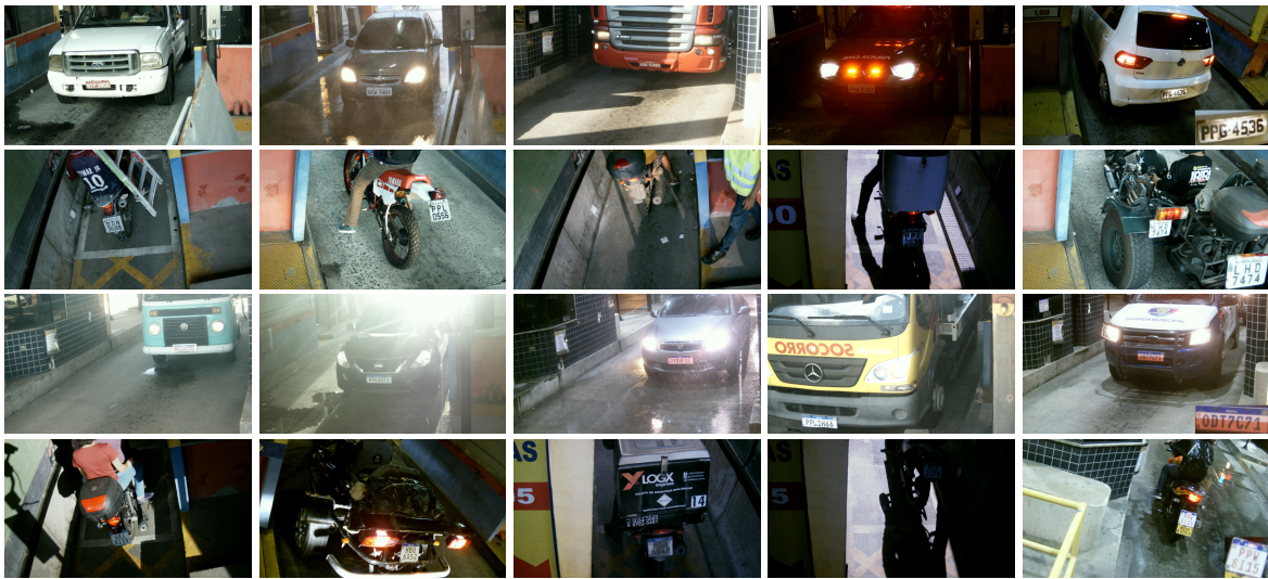
Figure 4.1: Some images extracted from the RodoSol-ALPR dataset. The first and second rows show images of cars and motorcycles, respectively, with Brazilian LPs (i.e., the standard used in Brazil before the adoption of the Mercosur standard). The third and fourth rows show images of cars and motorcycles, respectively, with Mercosur LPs. We show a zoomed-in version of the vehicle’s LP in the lower right region of the images in the last column for better viewing of the LP layouts. All human faces were blurred in every image due to privacy constraints.
