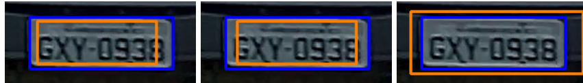
Figure 3.3: Three LPs detected with the same IoU value (0.7) with the ground truth; however, only the rightmost has all LP characters completely visible. The ground truth bounding boxes are outlined in blue, while the hypothetical predictions are outlined in orange. Image reproduced from (Gonçalves et al., 2018).
