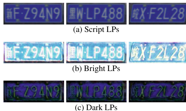
Figure 3.20: Zhang et al. (2019b) trained multiple CycleGAN-based networks (Zhu et al., 2017b) to generate LP images with different characteristics (b) (c). Each network was trained using script images (a) as one domain and real images with specific characteristics as another domain. Image reproduced from (Zhang et al., 2019b).
