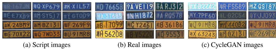
Figure 3.19: Wang et al. (2017) trained CycleGAN (Zhu et al., 2017b) to generate images of Chinese LPs (c). The CycleGAN model was trained using images created by a script (a) (i.e., colors and character deformations were hard-coded) as one domain and real images (b) as another. Image reproduced from (Wang et al., 2017).
