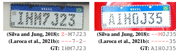
Figure 3.30: Recognition results yielded by two instances of the CR-NET model, one trained by Silva and Jung (2018) and the other by Laroca et al. (2021b), on two images of Mercosur LPs acquired by handheld cameras. For this evaluation, we used the weights provided by the respective authors in the supplementary material of each work.
