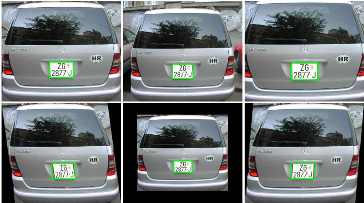
Figure 4.9: New training samples for LP detection and layout classification created using data augmentation. The upper-left image uses the ideal bounding box of the vehicle and the others were generated by adding some margin to it and through rescaling and shearing. The original image was taken from the EnglishLP dataset [109].
