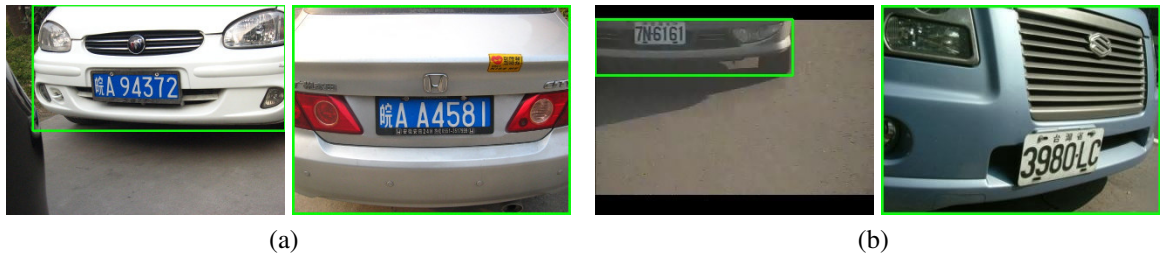
Figure 4.6: Examples of images in which only part of the vehicle is visible. The ROI (i.e., the ground truth) used for training our network is shown in green. Observe that detectors trained only on ‘entire’ vehicles would probably fail in these cases. The images in (a) and (b) were taken from the ChineseLP [45] and AOLP [107] datasets, respectively.
