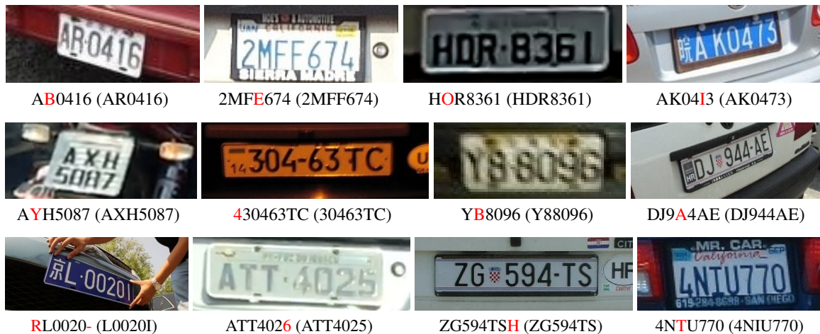
Figure 5.16: Examples of LPs that were incorrectly recognized by the proposed ALPR system. The ground truth is shown in parentheses.
