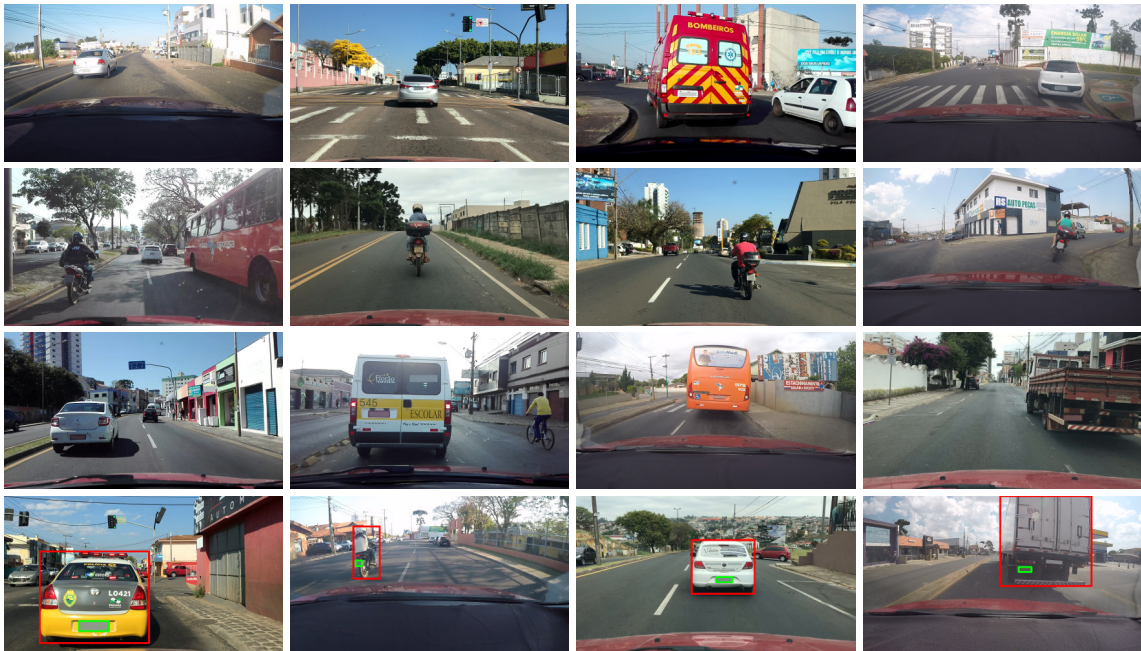
Figure 4.1: Sample images of the UFPR-ALPR dataset. First three rows show the variety in backgrounds, lighting conditions, as well as vehicle/LP positions and types. The 4th row shows examples of vehicle and LP annotations. The LPs were blurred due to privacy constraints.
