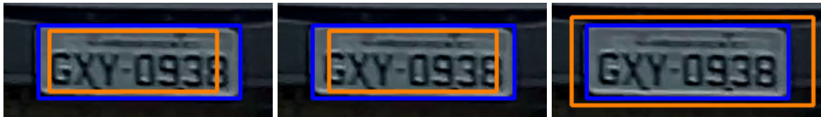
Figure 3.2: Three LPs detected with the same IoU value with the ground truth. Even at a high IoU threshold, it is not possible to guarantee that the detected LP encloses all characters. The ground truth bounding boxes are shown in blue and the hypothetical predictions are shown in orange. All three predictions have \text{IoU} = 0.7 with the ground truth, however, only the rightmost has all LP characters completely visible. Images reproduced from [13].
