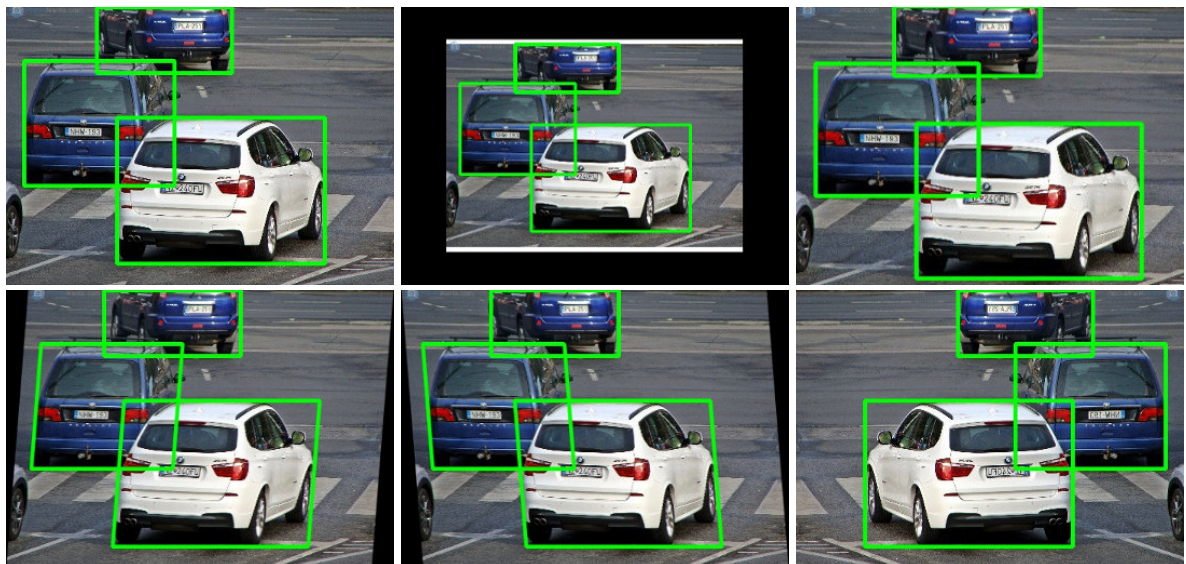
Figure 4.7: New training samples for vehicle detection created using data augmentation strategies. The upper-left image is the original (taken from http://platesmania.com/ ) and the others were generated through rescaling, shearing and horizontal flipping.
