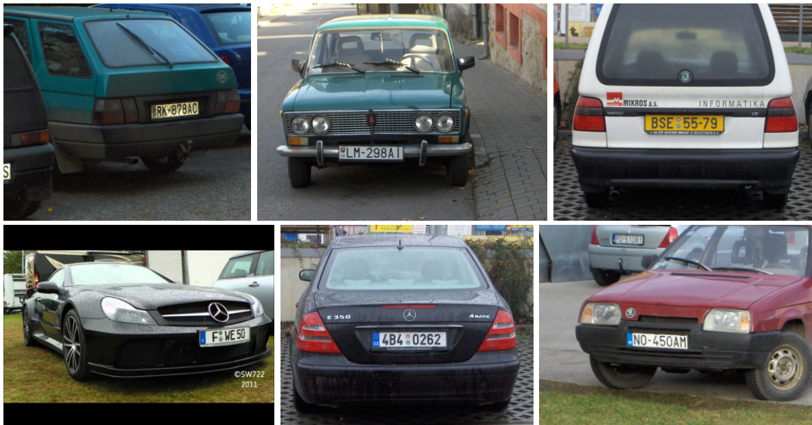
Figure 5.6: Some images from the OpenALPR-EU dataset [46]. In general, the vehicle occupies a large portion of the image and is well centered. Although in some cases there are legible LPs of other vehicles in the background (e.g., the bottom right image), only the position and text of the LP in the foreground are labeled in this dataset.
