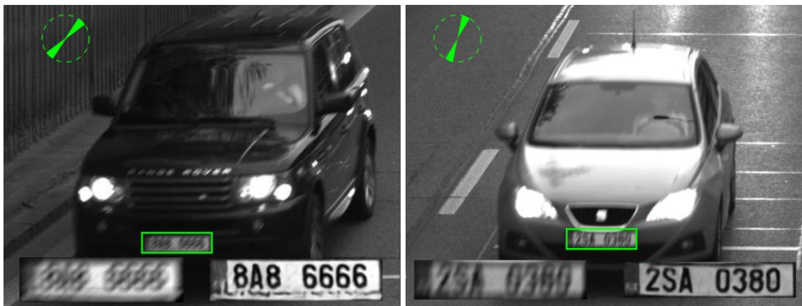
Figure 3.8: Blurred LPs captured by surveillance cameras and their respective reconstructions based on direct CNN deblurring. The network was trained for specific viewpoints using artificial data. Image reproduced from [101].
