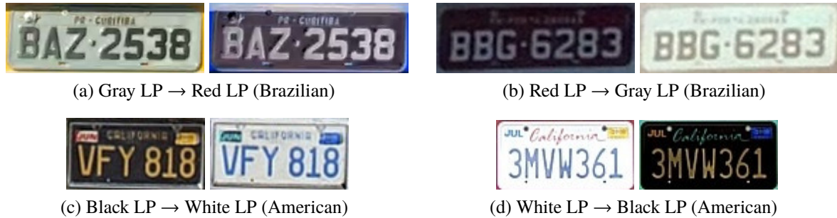
Figure 4.12: Examples of negative images created to simulate LPs of other layouts. (a) and (b) show Brazilian LPs, while American ones are shown in (c) and (d). In Brazil, private vehicles have gray LPs, while buses, taxis and other transportation vehicles have red LPs. In the United States, old California LPs featured gold characters on a black background. Currently, they have blue characters on a white background.
