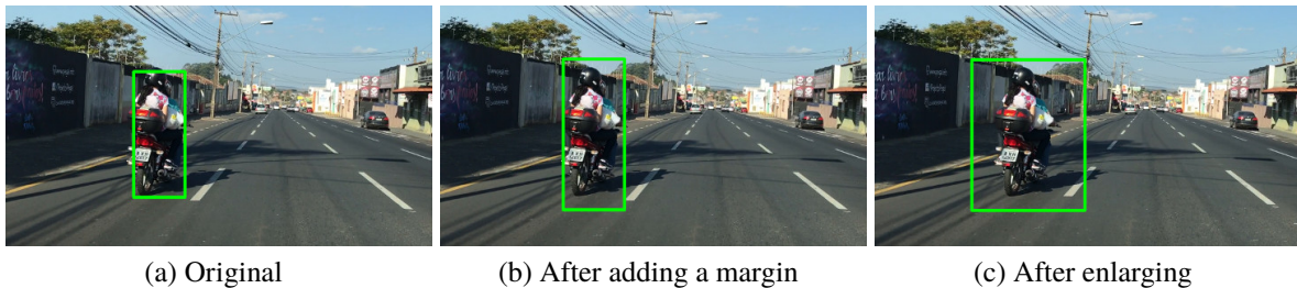
Figure 4.10: A vehicle’s bounding box after adding a small margin to it (10% of the size of the bounding box) and after enlarging it. In preliminary experiments, the results were better after (b) and worse after (c). In this way, we do not enlarge the vehicle patch after adding a small margin to it. This image belongs to the UFPR-ALPR dataset.
