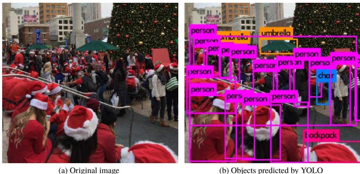
Figure 2.17: A limitation of YOLO. It might miss objects that are too close. In (a), there are 9 individuals in the lower-left corner, but only 5 were detected by YOLO, as can be seen in (b). Image reproduced from [71].
