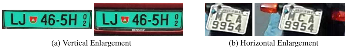
Figure 4.11: Two illustrations of enlargement of the LPs detected in the previous stage. In this way, a single network is trained to recognize LPs of different layouts, regardless of their aspect ratios. The LP patches in (a) and (b) were taken from the EnglishLP [109] and UFPR-ALPR datasets, respectively.
