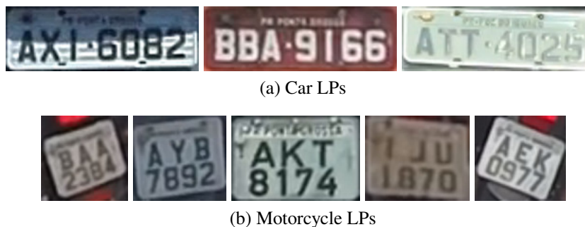
Figure 4.2: Examples of the LP layouts found in the UFPR-ALPR dataset. In Brazil, cars' LPs have 3 letters and 4 digits in the same row and motorcycles' LPs have 3 letters in one row and 4 digits in another.
