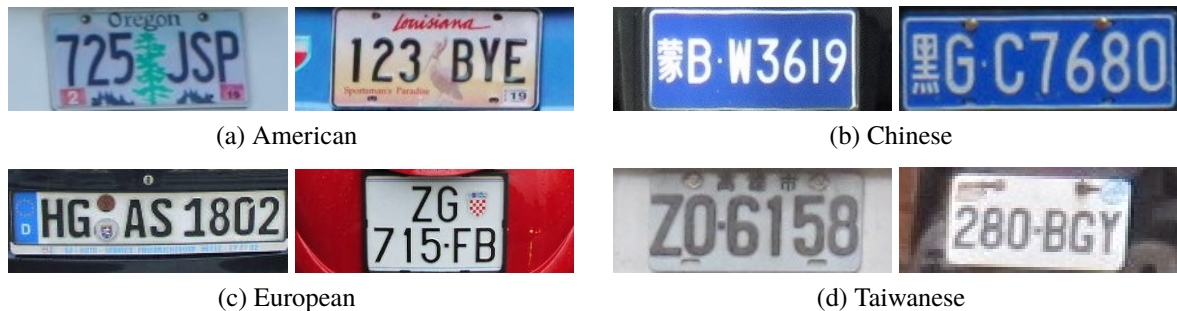
Figure 4.8: Examples of LPs of different layouts and classes. Observe the wide variety in different ways (e.g., aspect ratio, colors, symbols, position of the characters, number of characters, among others) on different LP layouts. The images in (a) and (b) were taken from http://platesmania.com/ , while the images in (c) and (d) are from the EnglishLP [109] and AOLP [107] datasets, respectively. Examples of Brazilian LPs are shown in Figure 4.2.
