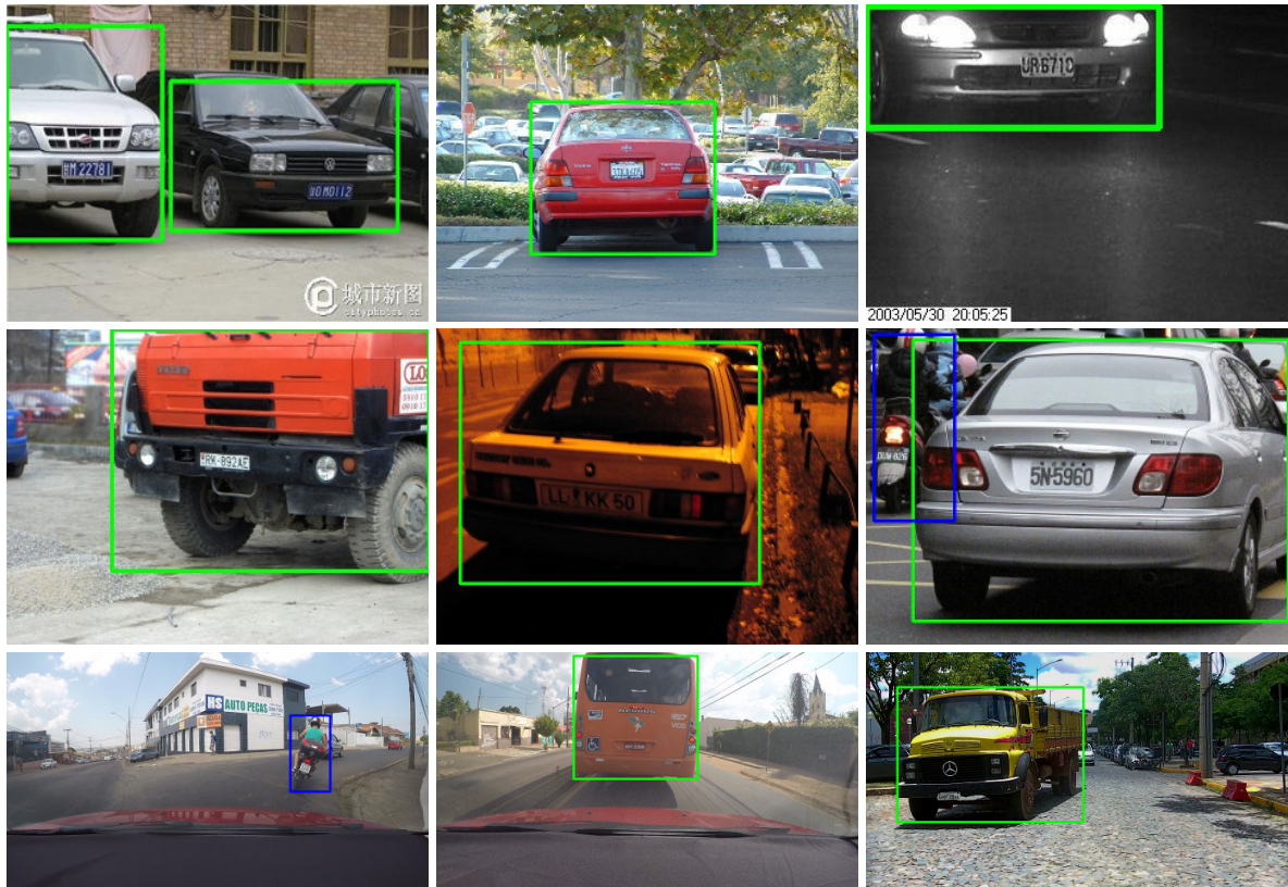
Figure 5.10: Some detection results achieved by the YOLOv2 model in different datasets. For better viewing, motorcycles' bounding boxes were drawn in blue, while the bounding boxes of other vehicles were drawn in green. Observe that vehicles of different types (cars, motorcycles, buses and trucks) were correctly detected regardless of lighting conditions (daytime and nighttime), occlusion, camera distance, and other factors.
