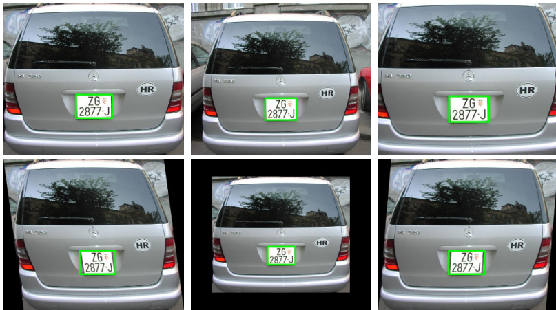
Figure 14: New training samples for LP detection and layout classification created using data augmentation.
