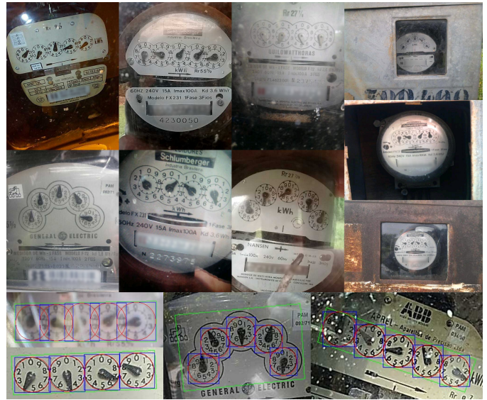
Fig. 2. Examples of the images chosen for the dataset. In the bottom row, there are examples of the annotations provided for each image: in green the irregular surrounding quadrilateral, in blue the bounding boxes around the dials and in red the maximal ellipse contained in the bounding box. Note that the customer meter identification is blurred for keeping subject privacy.
