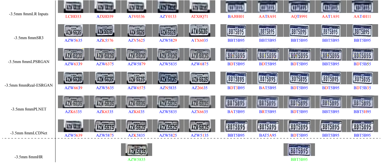
Figure 7. Recognition results for LPs cropped from images with a resolution of 1280 × 960 pixels. The top row shows the predictions made by GP_LPR [Liu et al., 2024b] on the original LR images, while the two subsequent rows present the predictions obtained from super-resolved images generated by PLNET [Nascimento et al., 2023, 2024a] and LCDNet [Nascimento et al., 2024b]. Below each image, the predicted characters are displayed, with correct characters highlighted in blue and incorrect characters in red. The ground truth is indicated in green.
