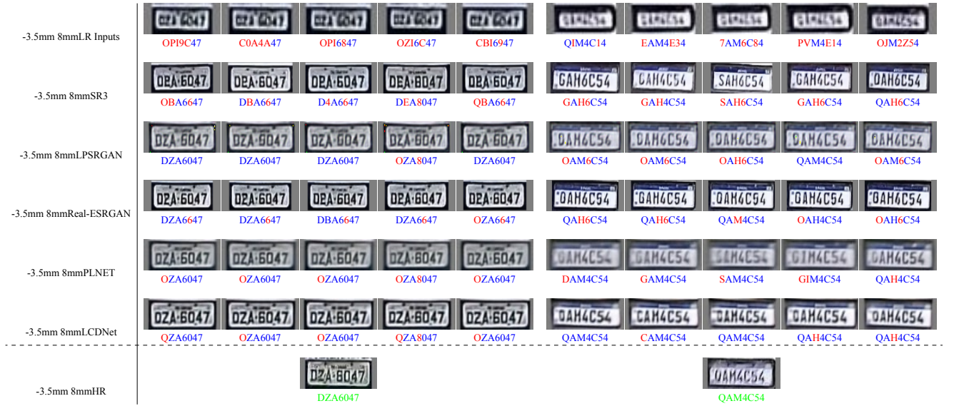
Figure 8. Recognition results for LPs cropped from images with a resolution of 1920 × 1080 pixels. The top row shows the predictions made by GP_LPR [Liu et al., 2024b] on the original LR images, while the two subsequent rows present the predictions obtained from super-resolved images generated by PLNET [Nascimento et al., 2023, 2024a] and LCDNet [Nascimento et al., 2024b]. Below each image, the predicted characters are displayed, with correct characters highlighted in blue and incorrect characters in red. The ground truth is indicated in green.
