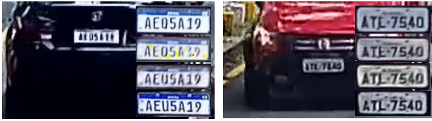
Fig. 4. Super-resolved LPs generated by our method and baselines from real-world images. The background image shows the original scene from which the LR image was extracted. From top to bottom: LP reconstructions by SR3 [35], PLNET [9], our method, and a reference HR image from a different frame.
