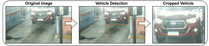
Fig. 3. Illustration depicting the process of extracting vehicle patches from images in the RodoSol-ALPR dataset, which lacks vehicle position labels.
