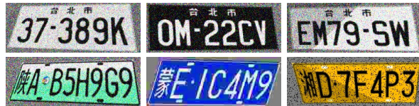
Fig. 4. Some of the many LP images we created to avoid overfitting. The images in the top row simulate LPs from vehicles registered in the Taiwan region (as in AOLP), while those in the bottom row simulate LPs from vehicles registered in mainland China (as in CCPD).
