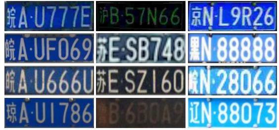
Fig. 2. Some Chinese LPs from the datasets used in our experiments. From top to bottom: CCPD [22], ChineseLP [30], PKU [31] and PlatesMania-CN [1]. The first character on each LP is a Chinese character representing the province in which the vehicle is affiliated. The second character is an English letter representing the city – in the province – in which the vehicle is affiliated [1].
