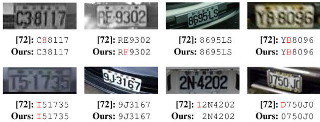
FIGURE 18 Some qualitative results obtained on the AOLP [61] dataset by Sighthound [72] and the proposed system
