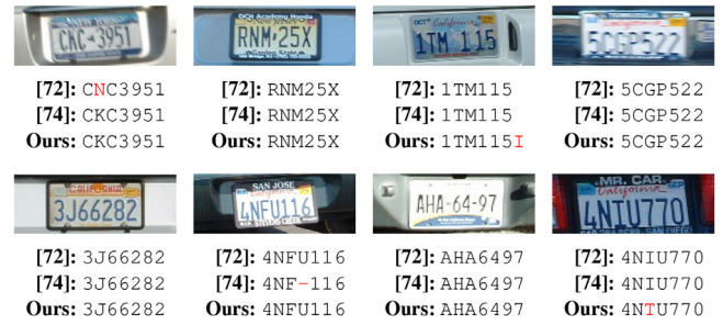
FIGURE 16 Some qualitative results obtained on UCSD-Stills [60] by Sighthound [72], OpenALPR [74] and the proposed system
