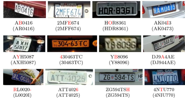
FIGURE 13 Examples of LPs that were incorrectly recognized by the proposed ALPR system. The ground truth is shown in parentheses
