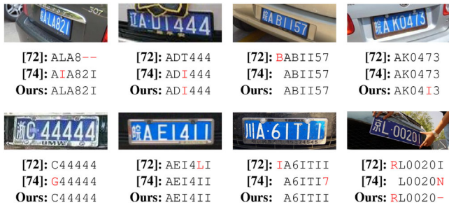
FIGURE 17 Some qualitative results obtained on ChineseLP [31] by Sighthound [72], OpenALPR [74] and the proposed system
