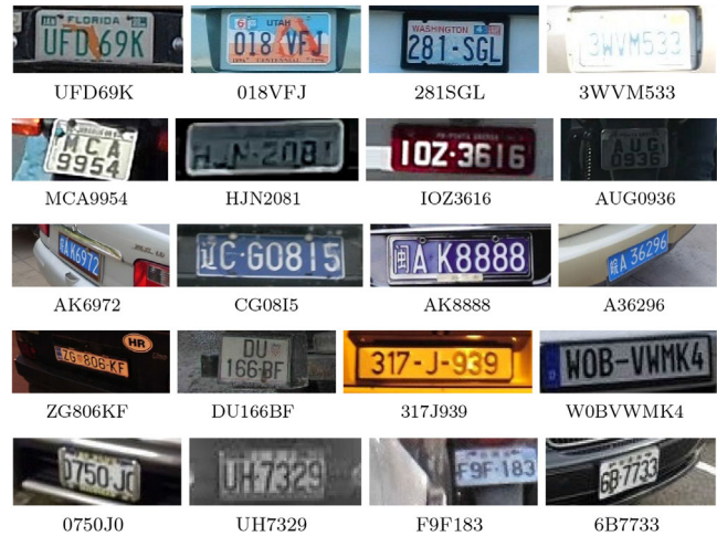
FIGURE 12 Examples of LPs that were correctly recognized by the proposed ALPR system. From top to bottom: American, Brazilian, Chinese, European and Taiwanese LPs
