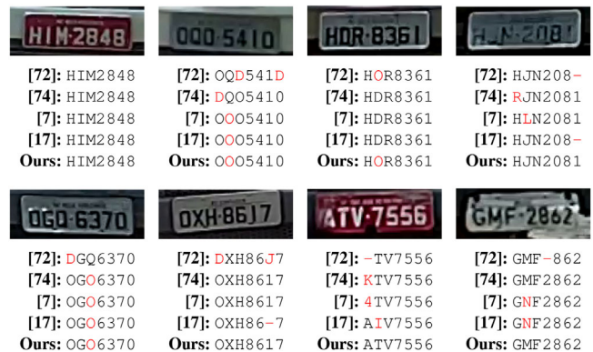
FIGURE 20 Some qualitative results obtained on SSIG-SegPlate [33] by Sighthound [72], OpenALPR [74], Silva and Jung [7], the preliminary version of our approach [17] and the proposed system
