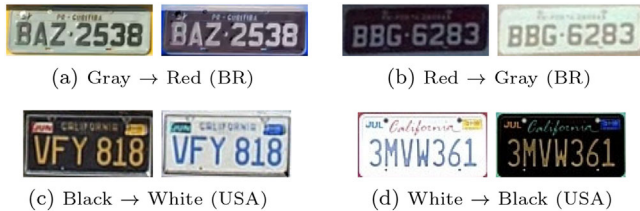
FIGURE 4 Examples of negative images created to simulate LPs of other layouts. In Brazil, private vehicles have grey LPs, while buses, taxis and other transportation vehicles have red LPs. In the United States, old California LPs featured gold characters on a black background. Currently, they have blue characters on a white background
