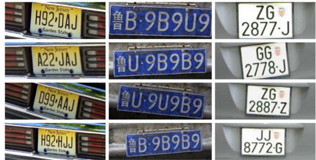
FIGURE 5 Examples of LP images generated by permuting the characters on the LPs. The images in the first row are the originals and the others were generated automatically
