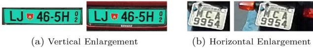
FIGURE 3 Two illustrations of enlargement of the LPs detected in the previous stage. In this way, a single network is trained to recognize LPs of different layouts, regardless of their aspect ratios
