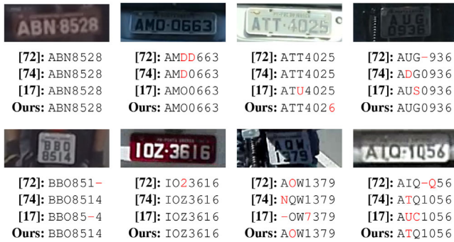
FIGURE 21 Some qualitative results obtained on UFPR-ALPR [17] by Sighthound [72], OpenALPR [74], the preliminary version of our approach [17] and the proposed system
