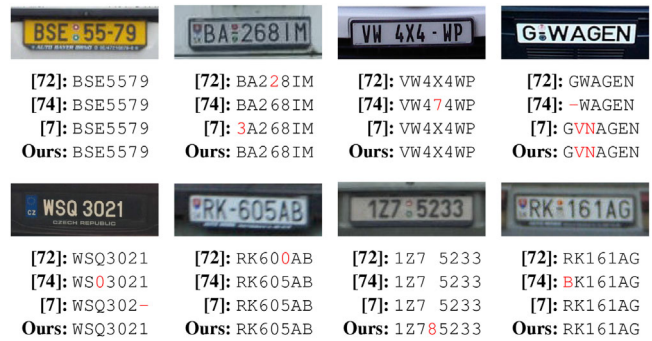
FIGURE 19 Some qualitative results obtained on OpenALPR-EU [32] by Sighthound [72], OpenALPR [74], Silva and Jung [7] and the proposed system
