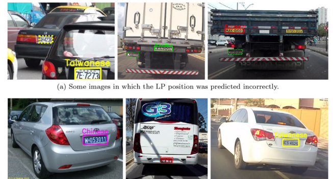
FIGURE 11 Some images in which our network failed either to detect the LP or to classify the LP layout
