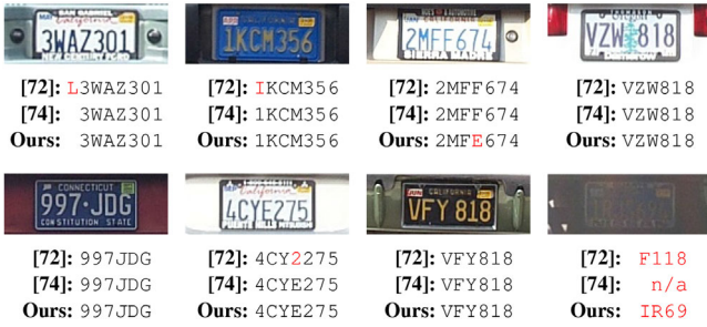
FIGURE 14 Some qualitative results obtained on Caltech Cars [58] by Sighthound [72], OpenALPR [74] and the proposed system
