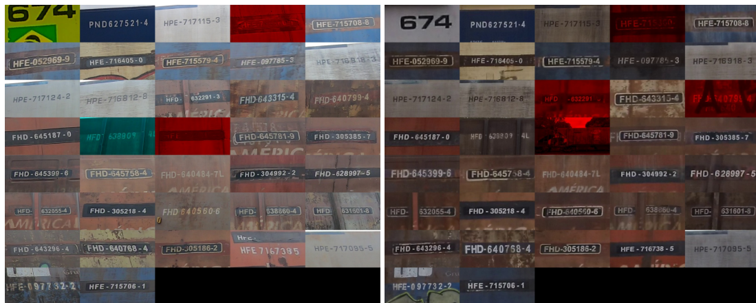
Figure 9. Mosaics of the same train composition recorded by two cameras, one on each side of the track.
