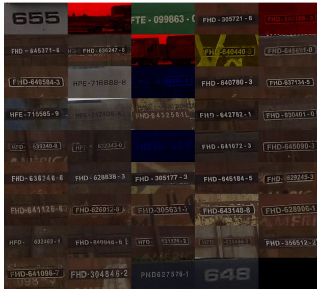
Figure 7. Mosaic generated automatically by the system after a train passes the control point where the camera is installed.
