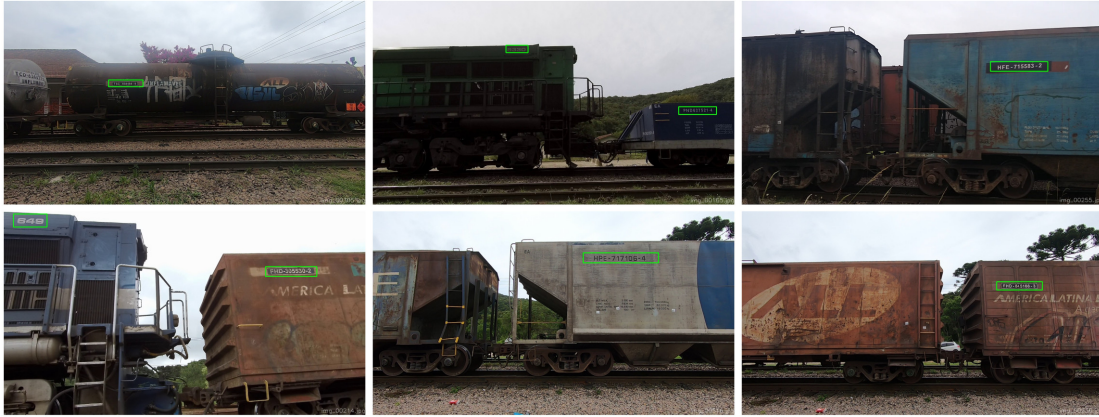
Figure 3. Examples of the detection results obtained for the wagon counting task.
