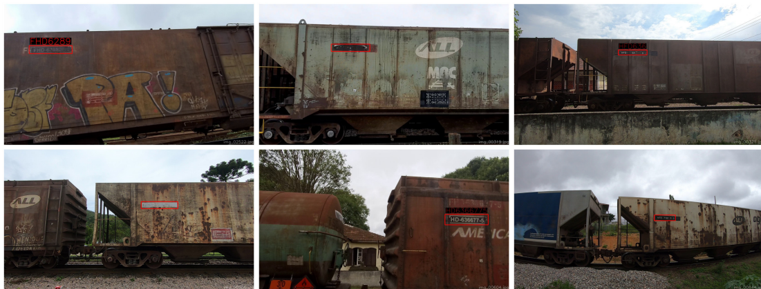
Figure 5. Examples of damaged/illegible identification codes.
