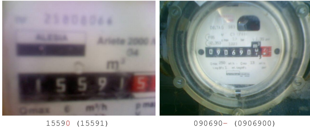
Fig 10 Incorrect readings obtained with the Fast-YOLO & CR-NET approach, where the last digit was incorrectly classified (left), and the last digit was detected/recognized with a confidence value below the threshold (right).
