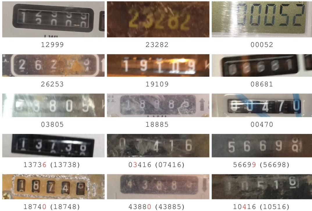
Fig 9 Results obtained by the CR-NET model in the UFPR-AMR dataset. The first three rows show examples of successfully recognized counters, while the last two rows show samples of incorrectly recognized counters. Some images were slightly resized for display purposes.
