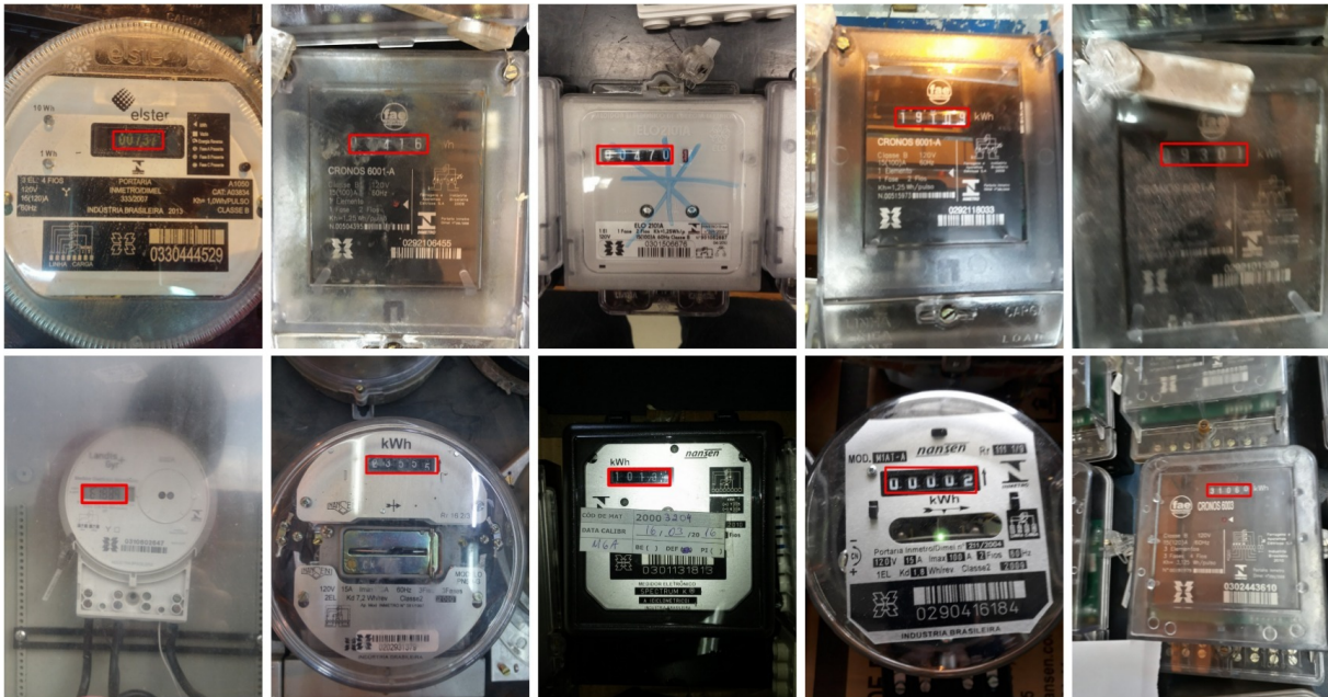
Fig 6 Samples of counter detection obtained with the Fast-YOLO model in the UFPR-AMR dataset.
