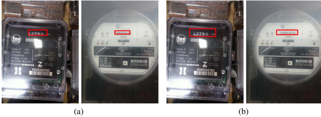
Fig 5 Bounding boxes predicted by the Fast-YOLO model before (a) and after (b) adding the margin (20% of the bounding box size).
