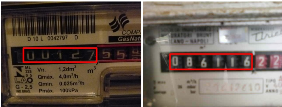
Fig 7 Examples of counter detection obtained with the Fast-YOLO model. Note that the counter region in the images of the Dataset 13 (left) and Dataset 5 (right) is quite larger than in the UFPR-AMR dataset.
