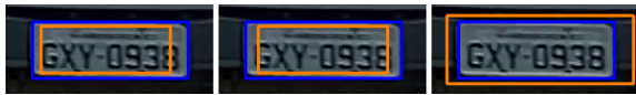
Fig. 2. The ground truth bounding boxes are shown in blue and hypothetical predictions are shown in orange. All three predictions have IOU = 0.7 with the ground truth, though only the rightmost has all seven characters completely visible.
