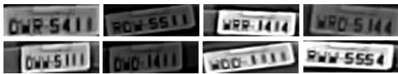
Fig. 4. Permutations of the same license plate. The top-left image is the original and the others were automatically generated.
